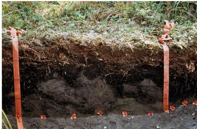
Figure 1: A shallow soil pit with a face that has been cleaned and prepared for describing the soil profile. This soil (a Fibristel in Alaska) has been dug to the depth of permafrost (about 40 cm).
