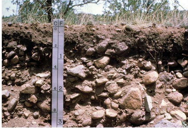
Figure 8: A soil in which the layers below a depth of about 20 cm are very cobbly loamy sand. Left side of scale is in 20-cm increments.
